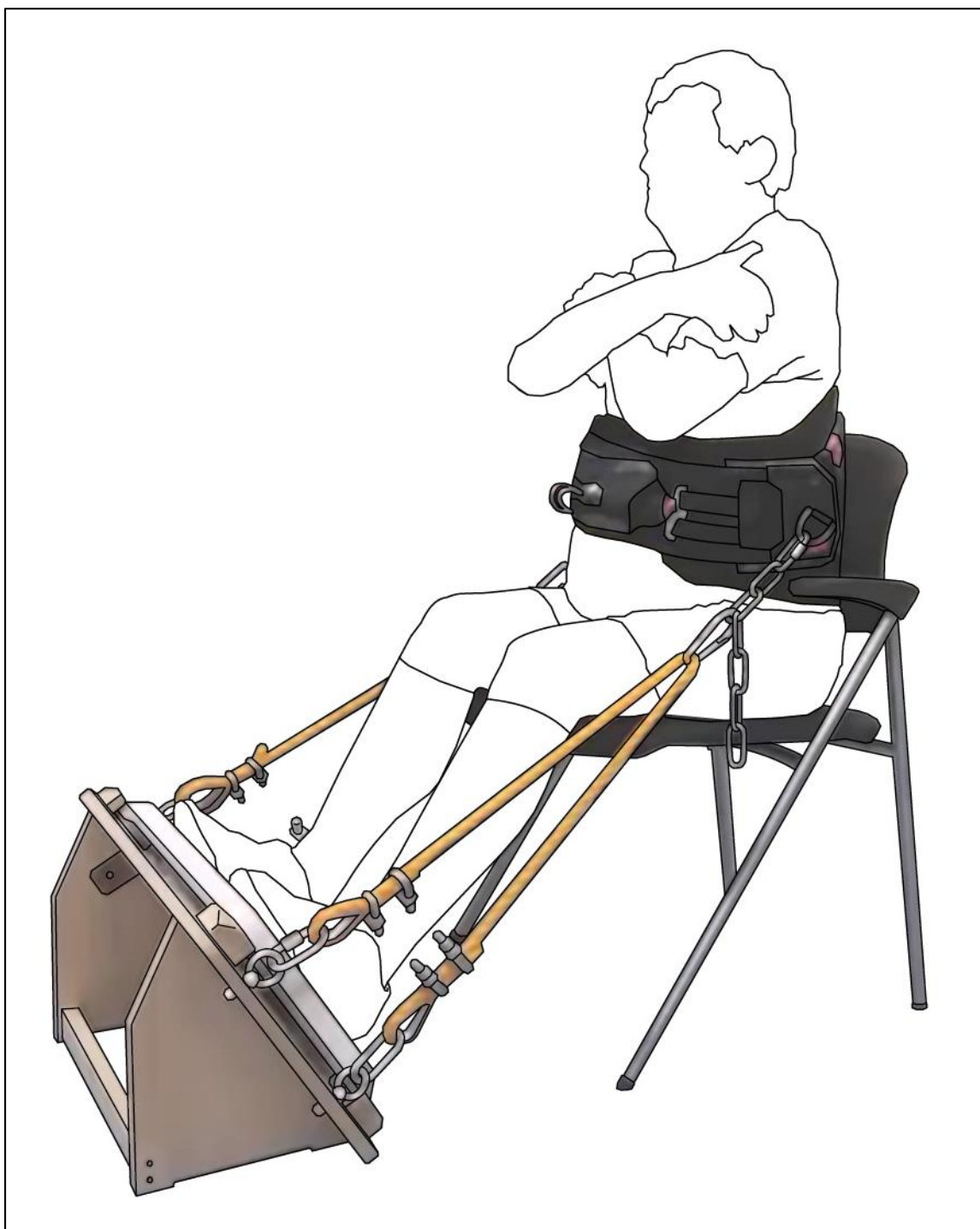
Supplementary file 6. Leg strength test on force plate (mod. Nintendo Wii Balance Board) in custom build bracket.
